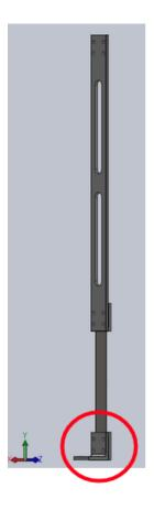
Install assembled flexure/vertical flexure support/corner bracket/bracket connector assembly to to flexure already installed onto pendulum top OK?\_\_\_\_\_
