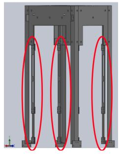
Fasten lower Corner Bracket (p/n-CB4) to support table(?) OK?\_\_\_\_\_
