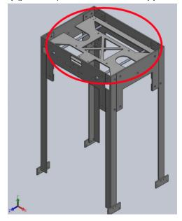
Install Pendulum 4 Corner Brackets(p/n-CB4) onto pendulum top
