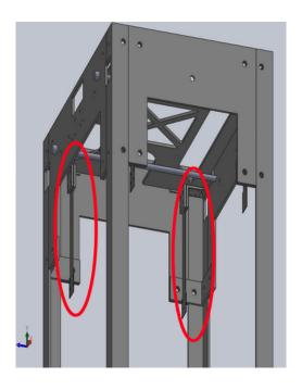
Install flexure to be tested onto vertical flexure support(p/n-VS1) using bracket connector (p/n-CB4) to clamp flexure in place OK?\_\_\_\_\_
